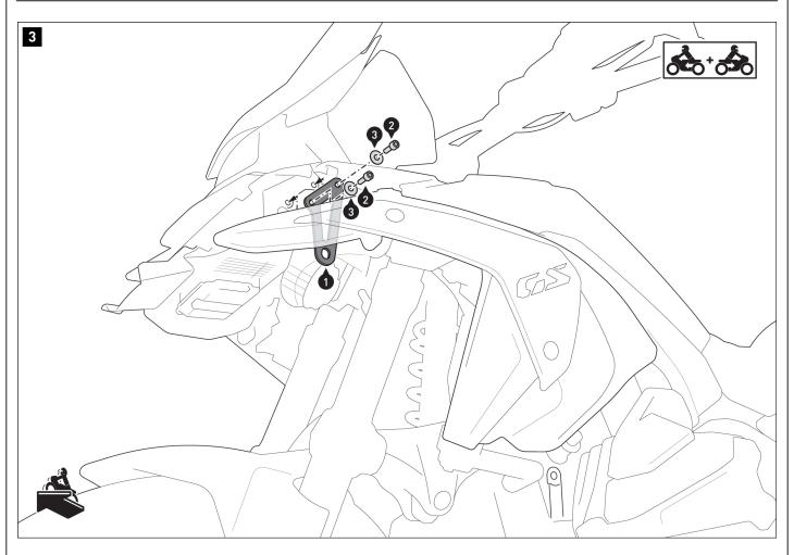
Screw the mounting brackets (1) onto both sides of the vehicle. Make sure to route the cables located at the mounting points past the mounting brackets on the inside.
