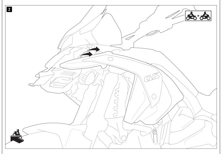
Remove the indicated screws from the vehicle on both sides.
