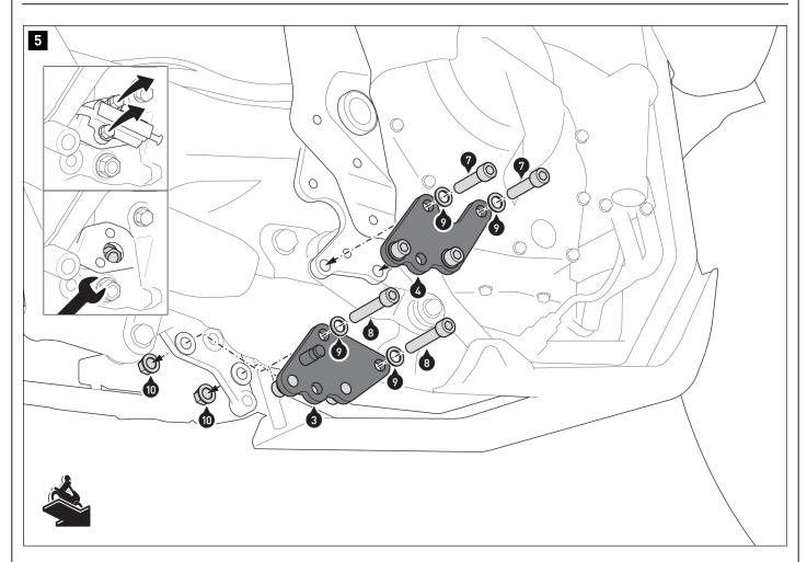
Loosen the side stand sensor on the left side of the vehicle to make it easier to mount the nut (10).
