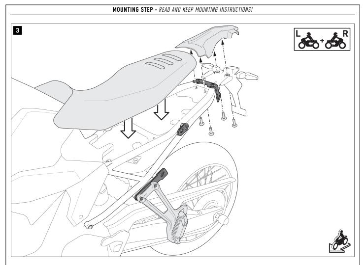
Attach the rear cover. Tighten the original screws according to the manufacturer's instructions.
