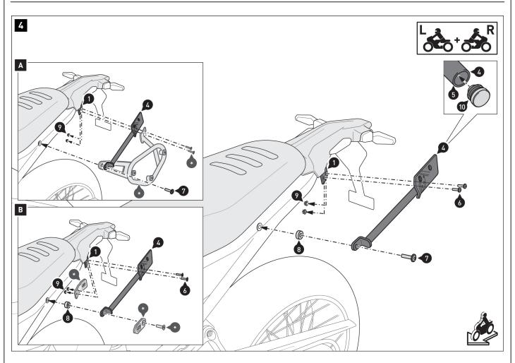
▲ **NOTE:** When installing at the same time as the SW-MOTECH SLC side carrier (\*), screw the parts together as shown in detailed drawing A. The spacer (8) and the screws (6) are no longer required. Instead, use the screws (\*) that come with the side carrier.
