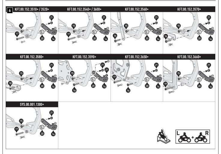
Screw the fastening tabs (14) and the attachment parts for your SW-MOTECH adapter kit to the mounting points shown on the side carriers (11/12). Please follow the mounting instructions for the SW-MOTECH adapter kit.
