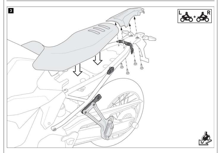
Attach the rear cover. Tighten the original screws according to the manufacturer's instructions.
