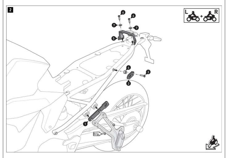
Screw the fastening tabs (1) to the passenger footrests **on both sides.**  $\triangle$  WARNING: Use liquid threadlocker! Do not tighten the original screws [Orig.] yet.
