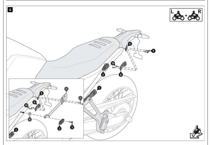
⚠ **NOTE:** If you are also installing the SW-MOTECH luggage rack (\*), screw the parts together as shown in the detailed drawing. The spacers (4) and screws (9) are not required in that case. Instead, use the spacers (\*) and screws (\*) included with the luggage rack.
