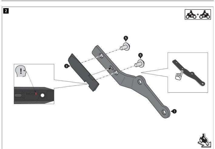
$\triangle$  **NOTE:** Screw the connector mounting rails (3/4) onto the side of the mounting brackets (1/2) marked in the picture.
