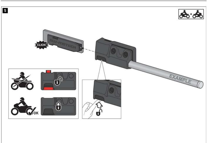
Slide the connectors (15/16) onto both sides of the connector mounting rails (3/4).
