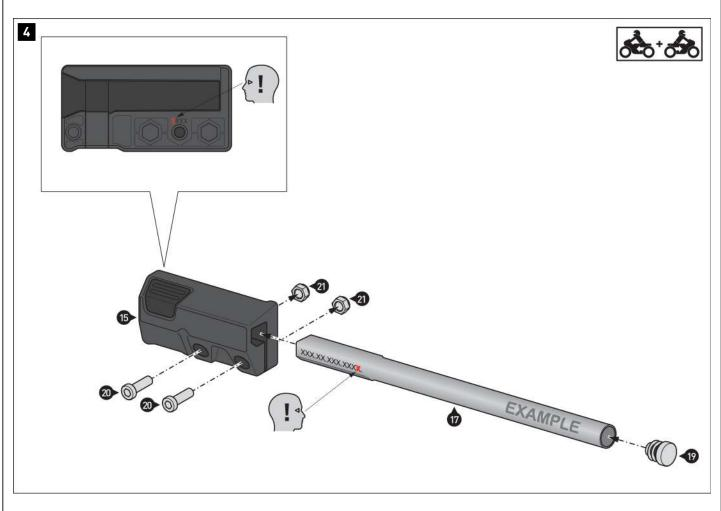
Insert the plastic plugs (19) into the ends of the support arms (17/18).
