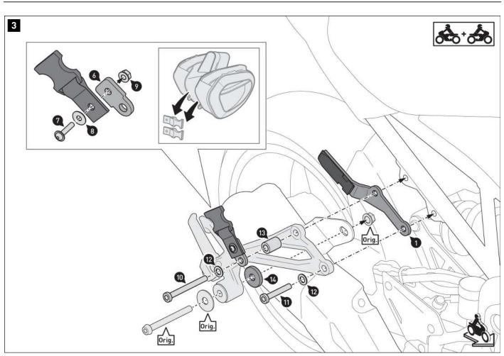
Remove the buckles (\*) from your saddlebags. Screw the buckles (\*) onto the mounting plates (6) as shown in the detailed drawing. Tighten the screws (7) as specified.
