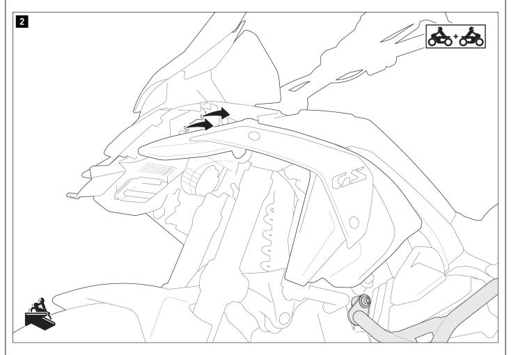
Remove the screws shown  ${\bf on\ both\ sides}$  of the vehicle.
