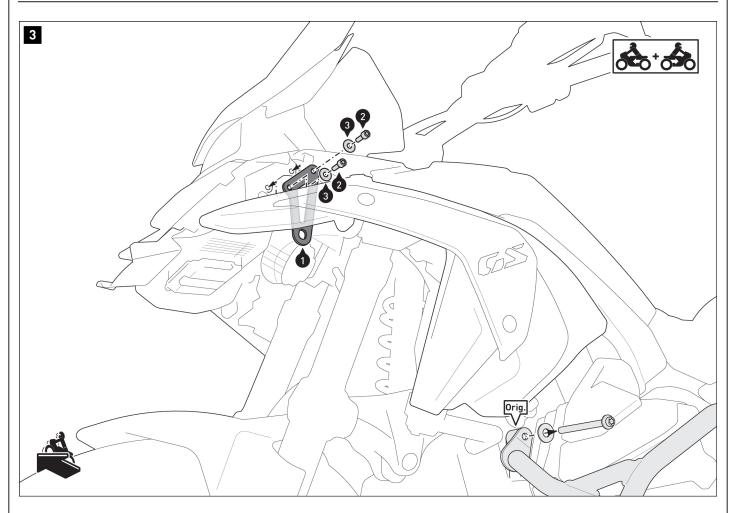
Screw the mounting brackets (1)  ${f onto}$  both sides of the vehicle. Make sure to route the cables located at the mounting points past the mounting brackets
