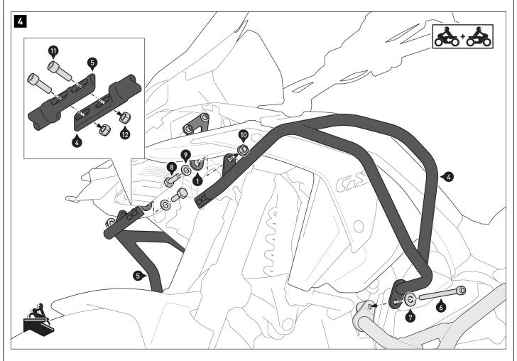
Screw the upper crash bars (4) and (5) on both sides to the original stainless steel crash bars on the vehicle and to the mounting brackets (1).
