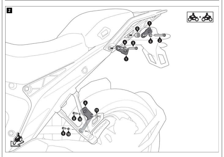
Screw in the fastening straps (1), (6), and (7) on both sides of the vehicle. **A WARNING:** Use a liquid threadlocker!
