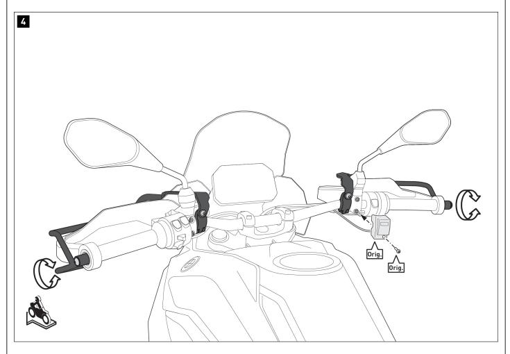
When all components are in place without tension, tighten the screws (4) as specified in the instructions.
