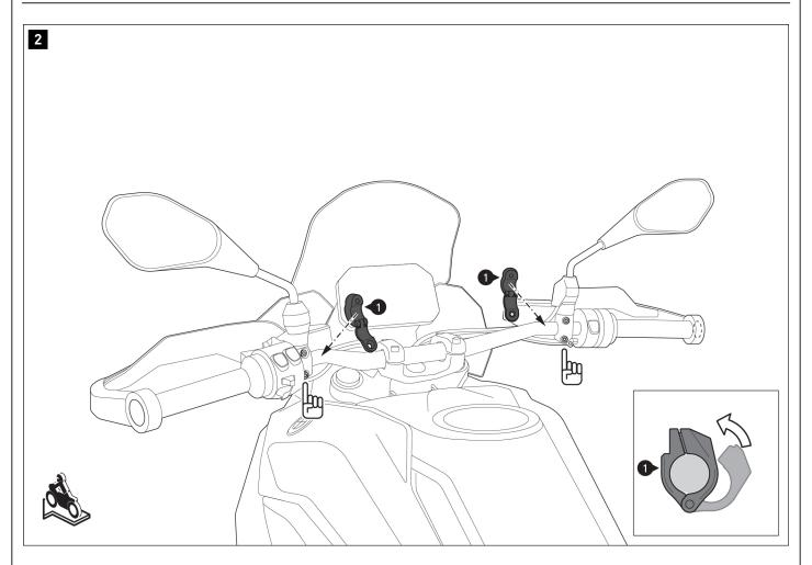
Place the two clamps (1) around the handlebars.
