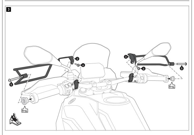
Screw the two hand protectors (2) and (3) to the original handlebar ends (orig.) on the vehicle.
