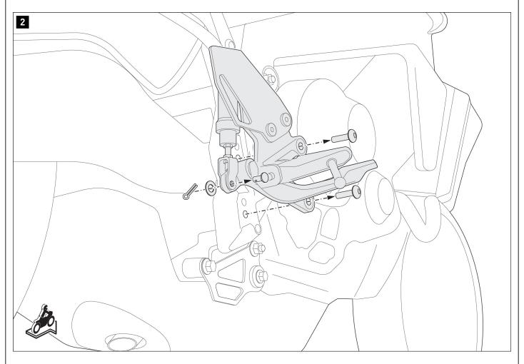
Remove the cotter pin and screws from the footpeg bracket.
