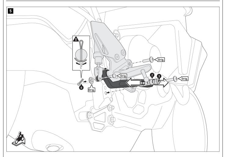
Screw the footpeg bracket to the vehicle using the original parts (Orig.).
