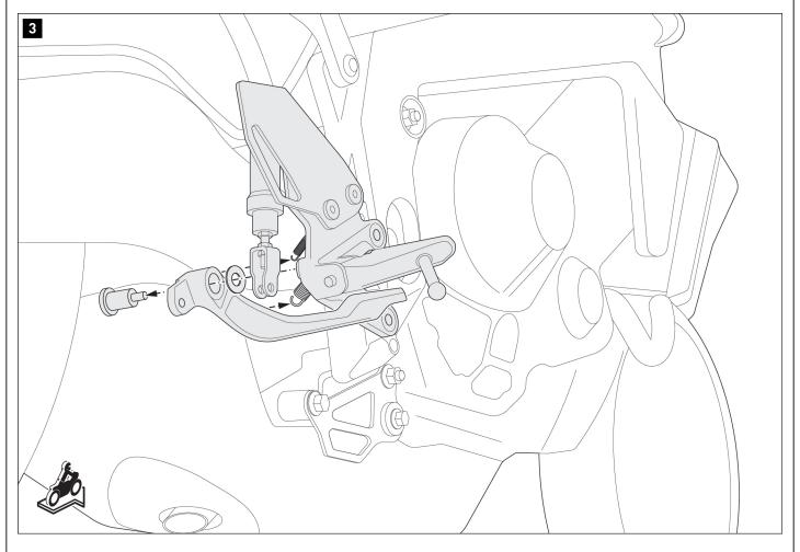
$\triangle$  **NOTE:** Before removing the original brake pedal, make a note of the Order and alignment of the original springs .
