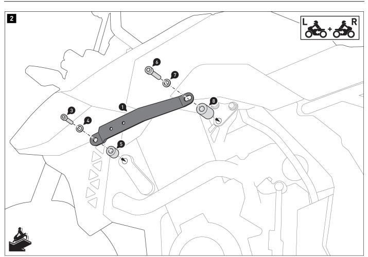
Screw the mounting brackets (1) onto the vehicle. **A WARNING: use liquid thread locker!** Tighten the screws (3) and (6) according to the manufacturer's instructions.
