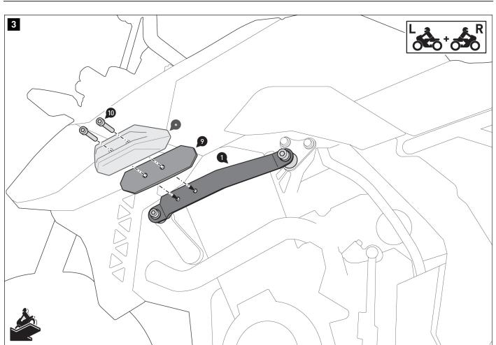
Screw the adapter plates (9) onto mounting brackets (1) & (2). **NOTE:**See also mounting instructions for the SW-MOTECH crash pad set (\*). **WARNING: Use a liquid threadlocker!** Tighten the screws (10) as specified in the mounting instructions.
