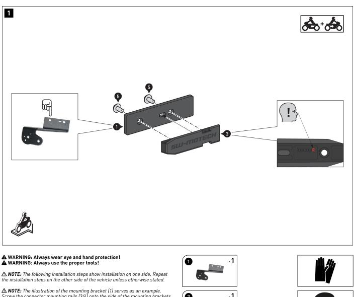
$\triangle$  **NOTE:** The illustration of the mounting bracket (1) serves as an example. Screw the connector mounting rails (3/4) onto the side of the mounting brackets (1/2) marked in the picture.
