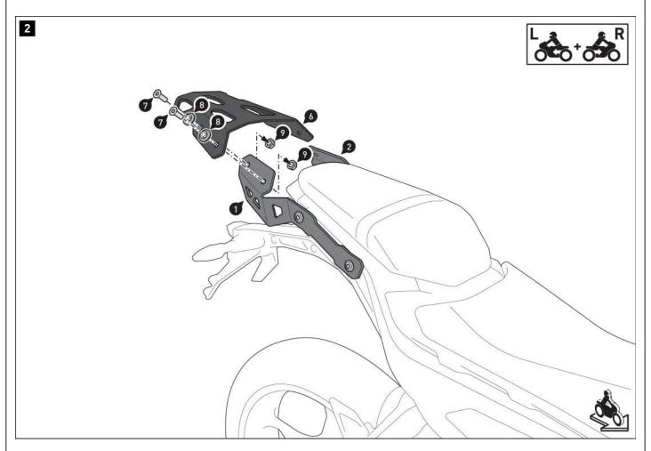
Screw the rack (6) onto the mounting brackets (1) and (2).
