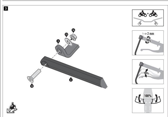
Screw the inner ends of the brackets (6/7) to the connecting plates (3/4). Do not tighten the screws (12) yet.
