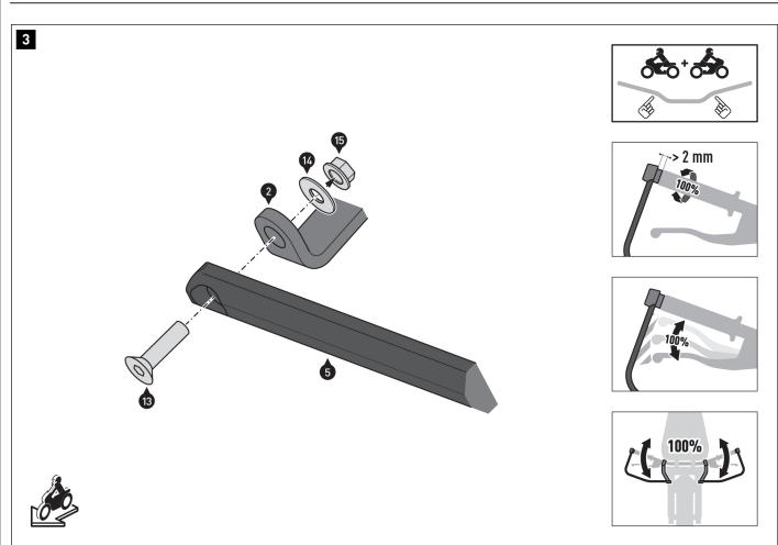
Screw the inner ends of the brackets (5/6) to the connecting plates (2/3). Do not tighten the screws (13) yet.
