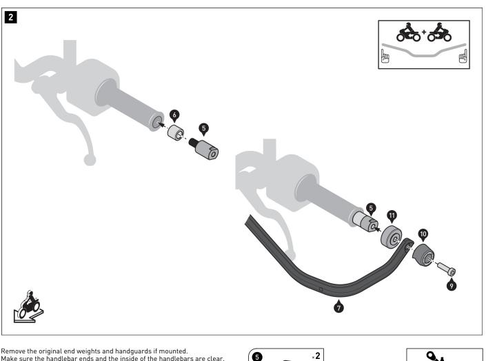
Remove the original end weights and handguards if mounted. Make sure the handlebar ends and the inside of the handlebars are clear.
