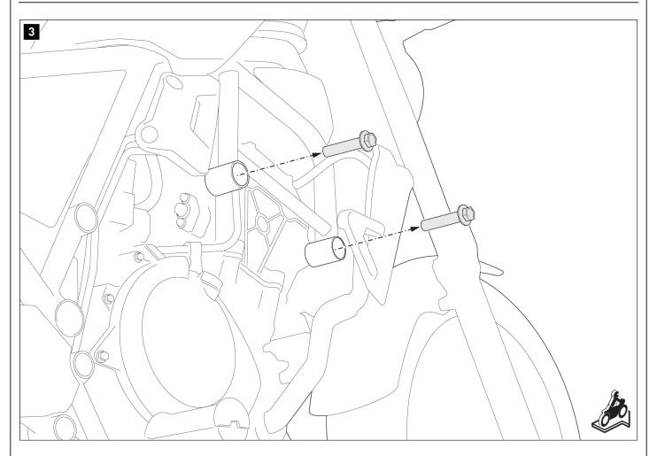
Remove the original parts from the  $\boldsymbol{right}$  mounting points.
