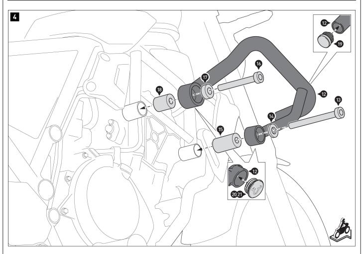
Insert the plastic plug (19) into the opening of the crash bar (12).
