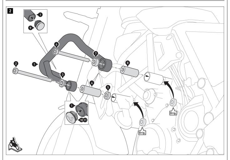
Insert the plastic plug (9) into the opening of the crash bar (1).
