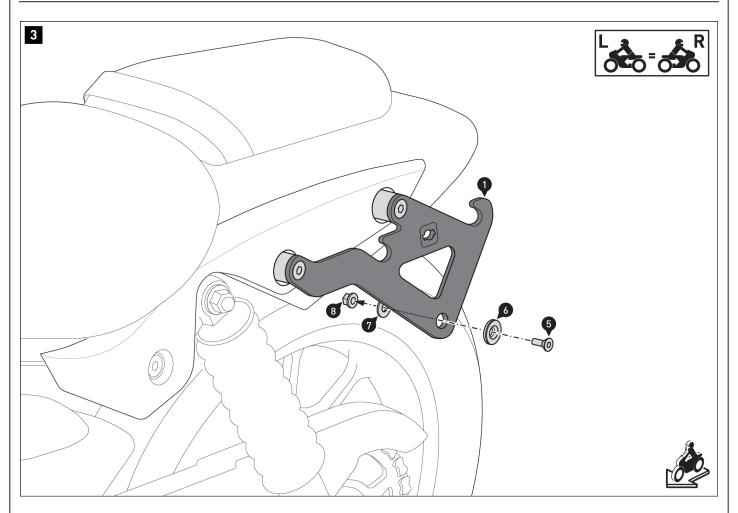
Screw parts (5) to (8) onto the side carrier (1). **A** WARNING: Use liquid threadlocker!
