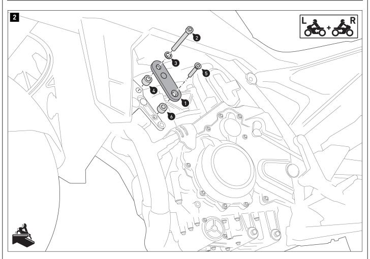
Screw the mounting brackets [1] onto the vehicle.
