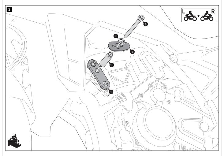
Screw the base plates (7) to the mounting brackets (1). Before tightening the screws (8), align the base plates according to the lines of the vehicle.
