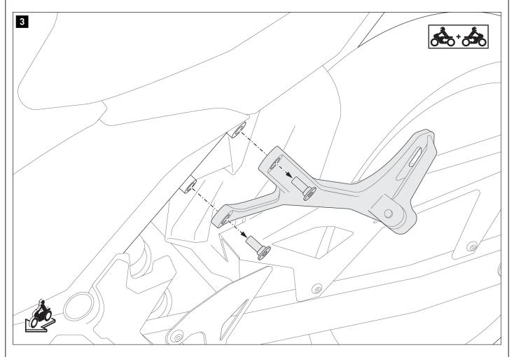
Remove the original parts shown  $\boldsymbol{from\ both\ sides}$  of the vehicle.
