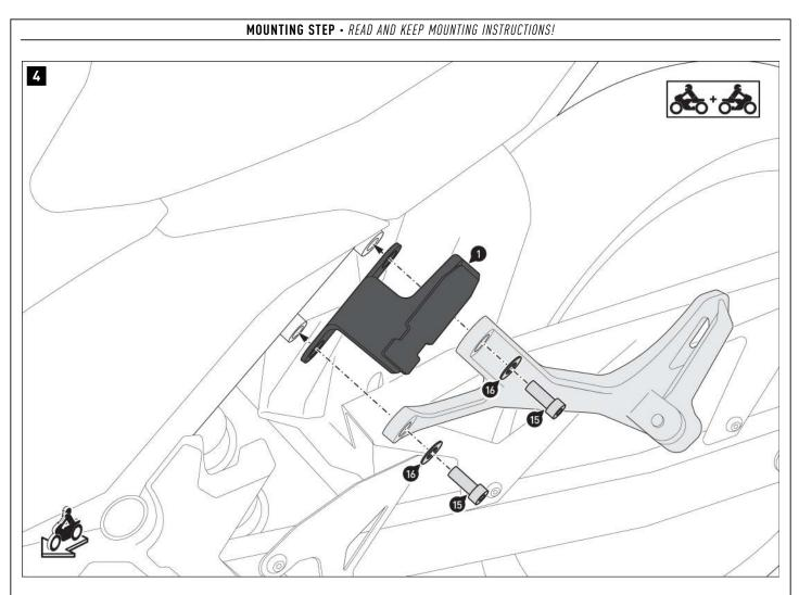
Screw the mounting brackets (1/2) onto the vehicle. **A WARNING: Use a liquid threadlocker!** Tighten the screws (15) according to the manufacturer's instructions.
