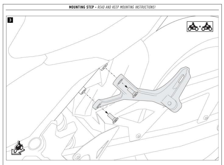
Remove the original parts shown **from both sides** of the vehicle.
