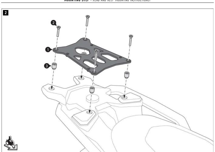
Screw the mounting bracket (1) to the mounting points shown. **A** WARNING: Use liquid threadlocker! Tighten the screws (2) according to the manufacturer's instructions.
