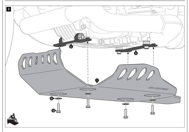
Screw the engine guard [1] to the mounting brackets (4) and [8]. **A WARNING:** Use a liquid threadlocker!
