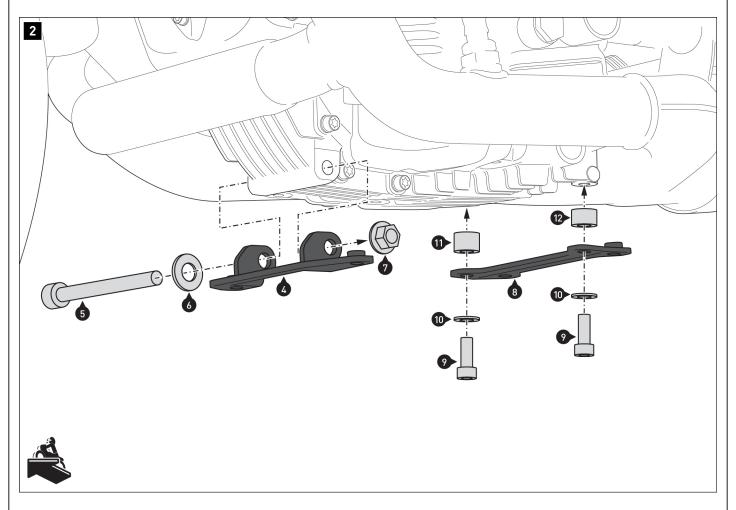
Screw the mounting brackets (4) and (8) to the vehicle.
