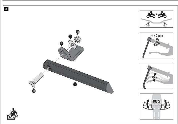
Screw the inner ends of the brackets (6/7) to the connecting plates (2/3). Do not tighten the screws (11) yet.
