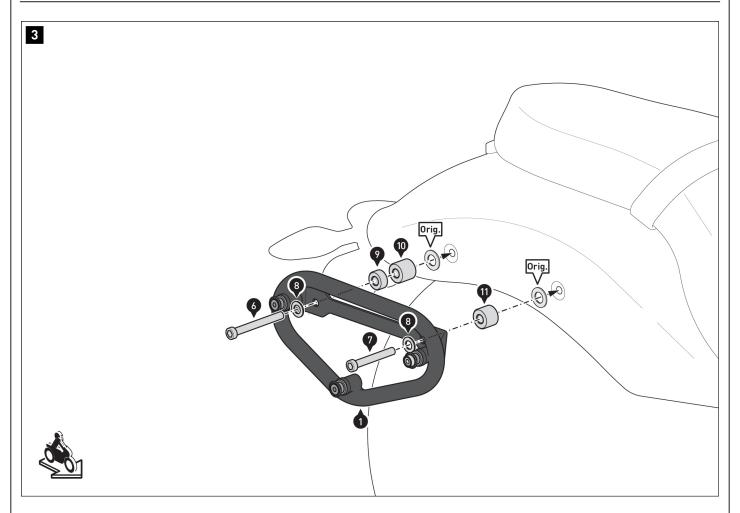
Screw the side carrier [1] to the vehicle using the original parts (Orig.) shown. **A WARNING:** Use a liquid threadlocker!
