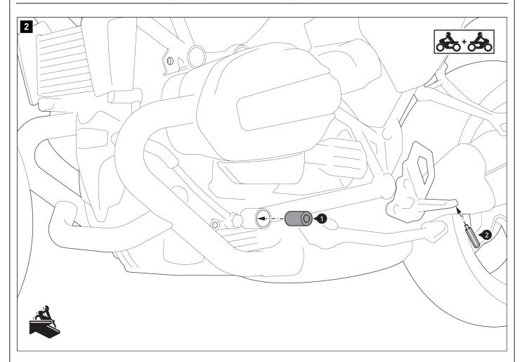
Insert the spacer (1) into the **left** frame opening.
