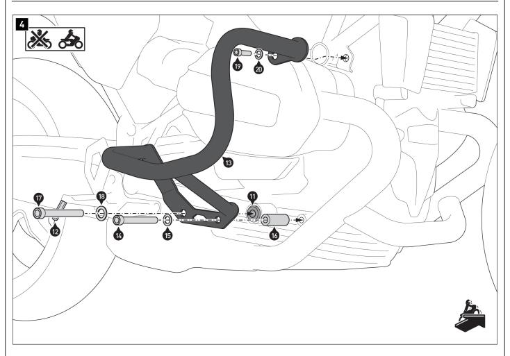
Remove the original engine mounting screw and the sliding sensor from the right side of the vehicle as shown in step [2].
