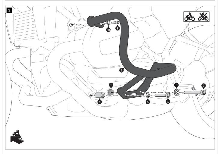
Screw the **left** crash bar [3] to the vehicle. **A WARNING:** Use a liquid threadlocker!
