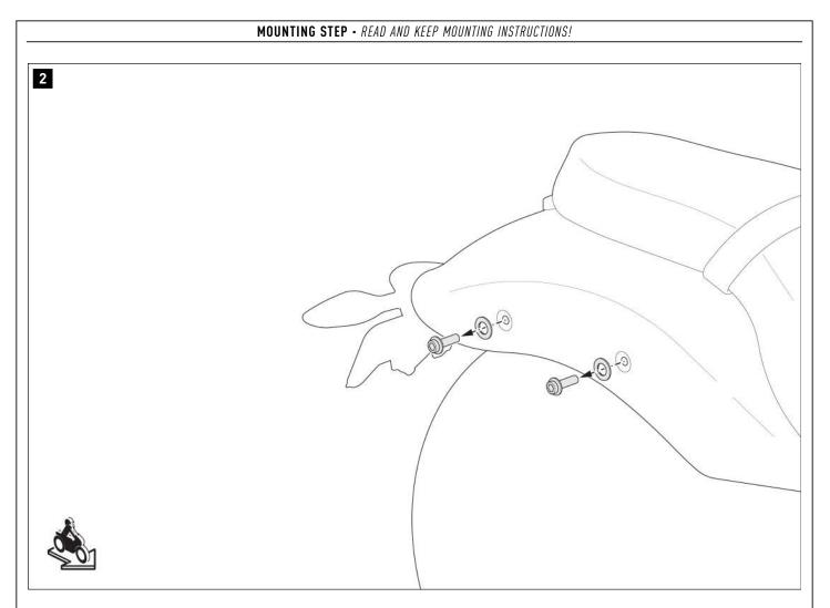
Remove the original screws shown from the vehicle.
