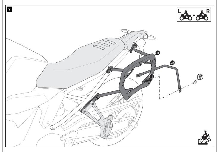
Use the the quick-release fasteners (13) to connect the crossbar (22) on both sides to the fastening tabs (14).
