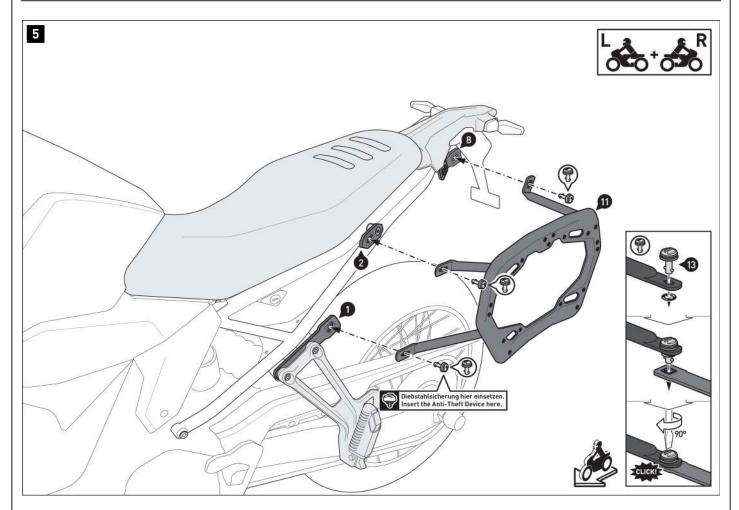
Connect the side carriers (11) and (12) on both sides with the quick-release fasteners (13) to the fastening tabs (1), (2) and (8).
