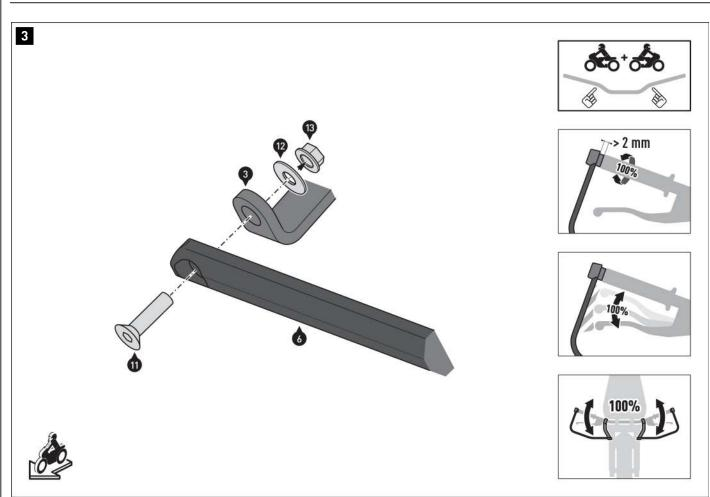
Screw the inner ends of the brackets (6/7) to the connecting plates (3/4). Do not tighten the screws (11) yet.
