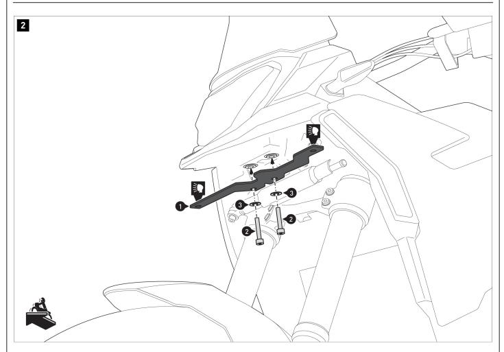
Screw the headlight mount [1] onto the vehicle.
