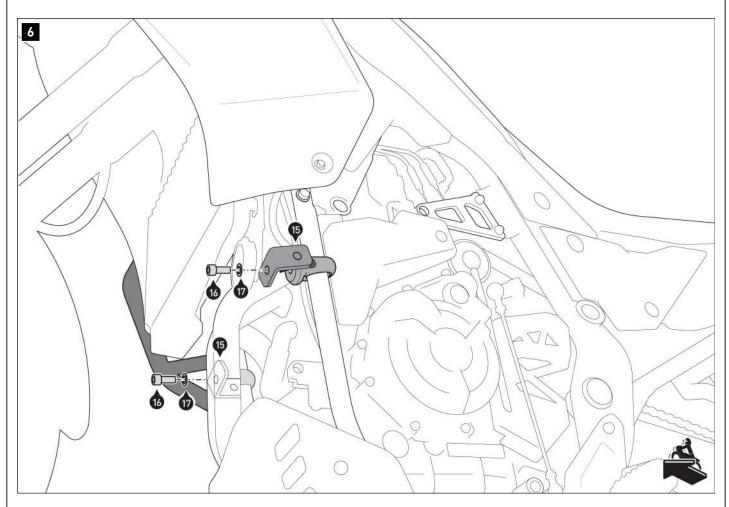
Screw the mounting brackets (15) onto clamps (1) and (12). **A WARNING:** Use a liquid threadlocker!
