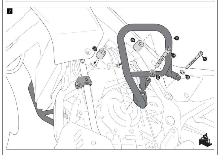
Screw the left crash bar (18) on to the vehicle. **A** WARNING: Use a liquid threadlocker!
