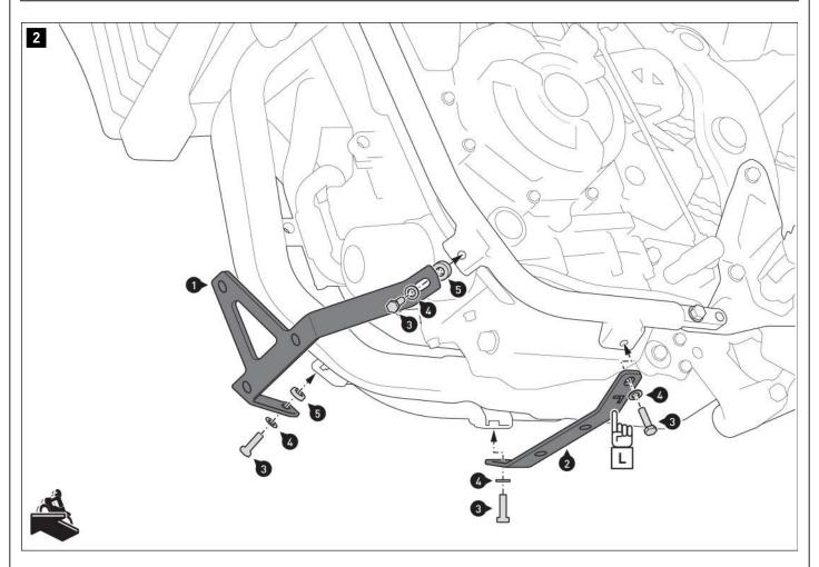
Screw the front (1) and middle (2) mounting brackets (L mark on the left side of the vehicle) to the vehicle frame.
