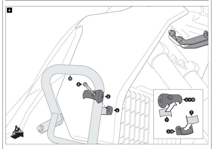
Glue the rubber strips (7) in clamps (5), (6), and (16) as well as in the clamps of the crash bars (9/10) as shown in the detailed drawing.
