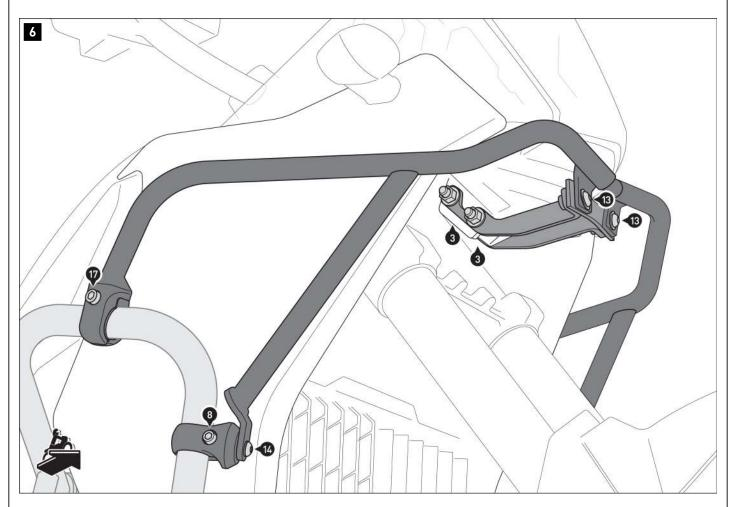
When all parts are seated without tension, tighten screws (3), (8), (13), (14) and (17) as specified in the mounting instructions.
