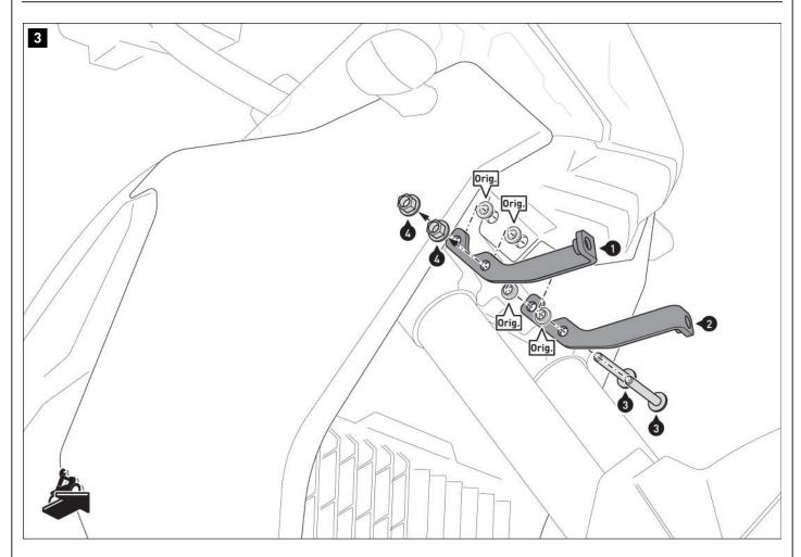
Screw the mounting brackets (1/2) onto the vehicle using the original spacers (Orig.). Do not tighten the screws (3) yet.
