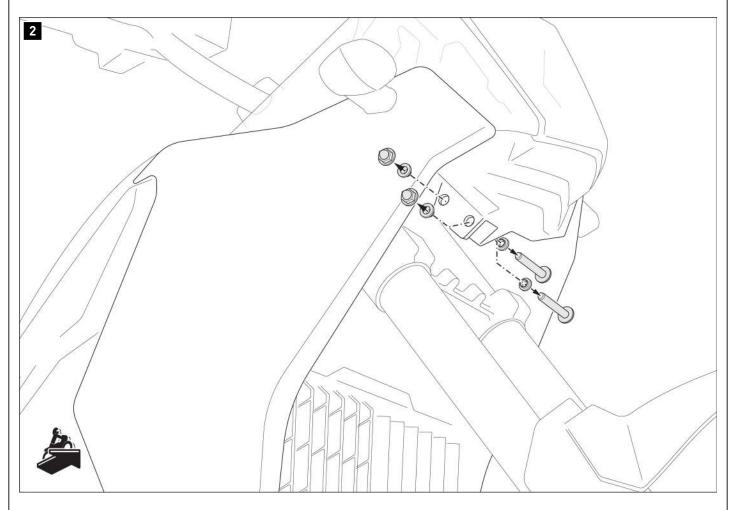
Remove the original parts from the attachment points shown.
