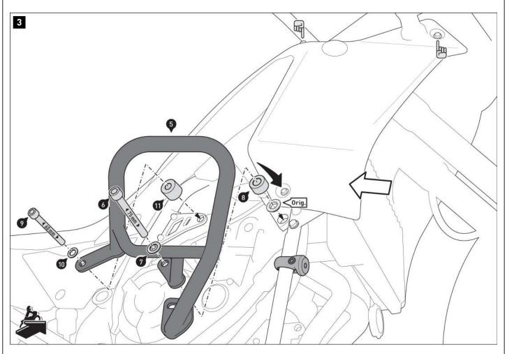
Screw the right crash bar (5) to the original socket (Orig.) on the vehicle. **A WARNING:** Use a liquid threadlocker!
