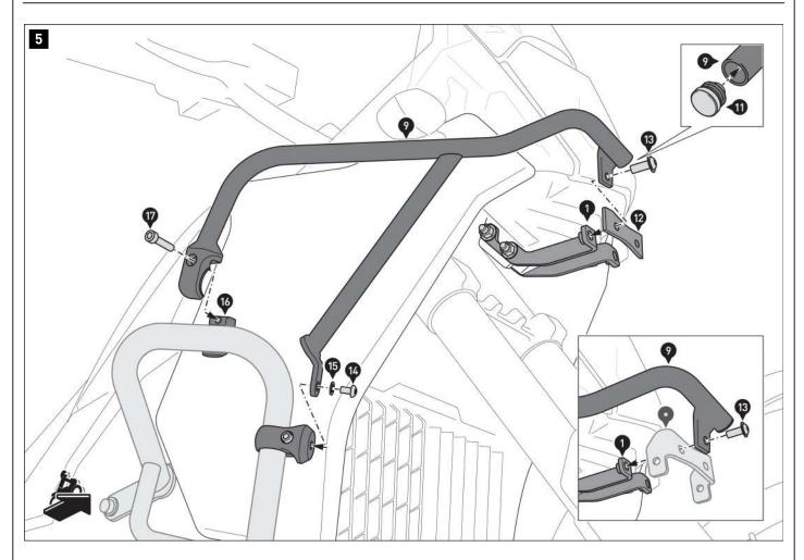
$\triangle$  **NOTE:** When installing the crash bar with the SW-MOTECH headlight holder, use the mounting bracket (\*) of the headlight holder as shown in the detailed
