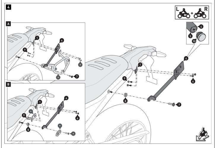
$\triangle$  **NOTE:** When installing at the same time as the SW-MOTECH SLC side carrier (\*), screw the parts together as shown in detailed drawing A. The spacer (8) and the screws (6) are no longer required. Instead, use the screws (\*) that come with the side carrier.
