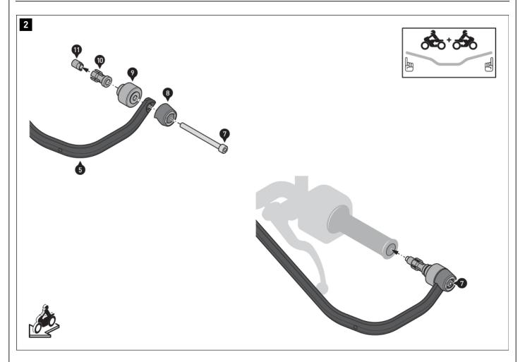
Remove the original end weights and handguards if mounted. Make sure the handlebar ends and the inside of the handlebars are clear.
