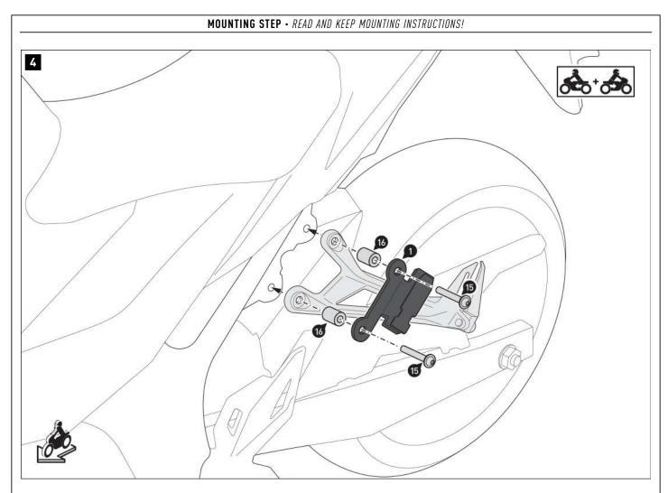
Screw the mounting bracket [1] to the vehicle. **A WARNING: Use a liquid threadlocker!** Tighten the screws (15) according to the manufacturer's instructions.
