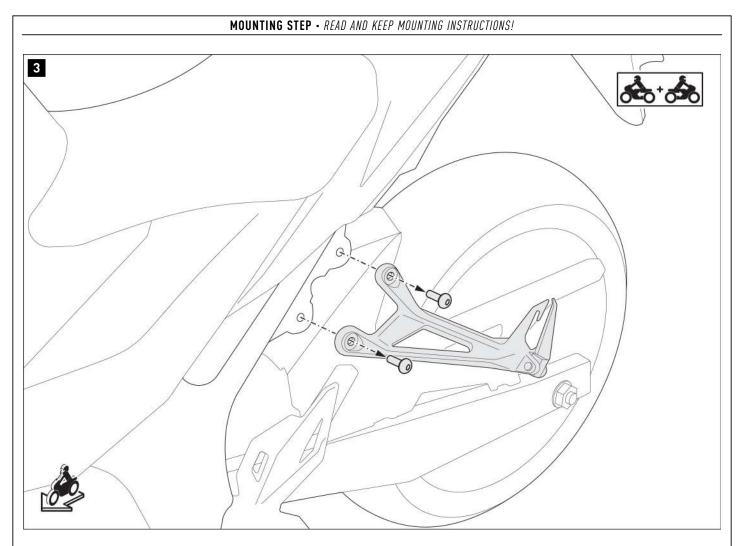
Remove the original parts shown here from the vehicle.
