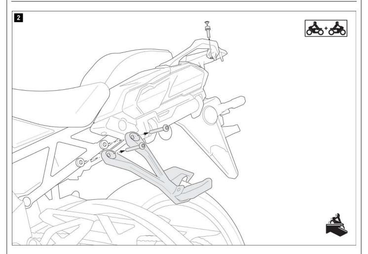
Remove the screws shown  ${\bf on\;both\;sides}$  and the passenger footrest holders from the vehicle.
