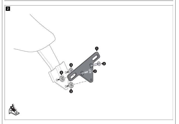
Screw the adapter plate (1) to the vehicle.
