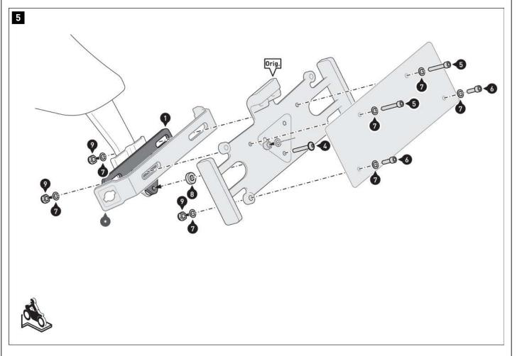
Screw the license plate, the license plate holder and the crossbar (\*) included with the SW-MOTECH side carrier to the parts shown on the adapter plate [1].
