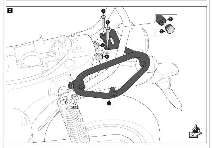
Insert the plastic plug (2) into the tube end of the side carrier (1).
