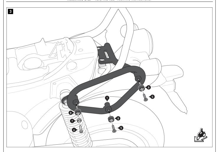
Screw parts (5) to (8) to the side carrier (1).
