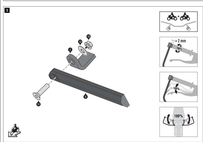
Screw the inner ends of the brackets (5/6) to the connecting plates (2/3). Do not tighten the screws (11) yet.
