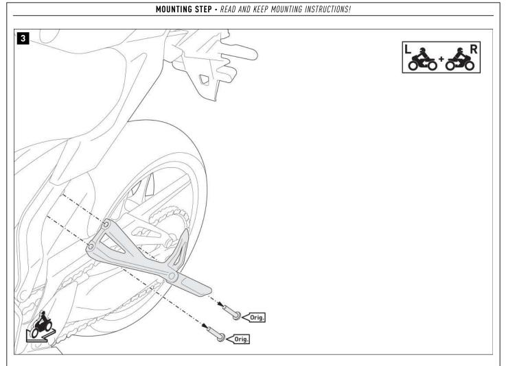
Remove the original parts shown  $\ensuremath{\textit{from both sides}}$  of the vehicle.
