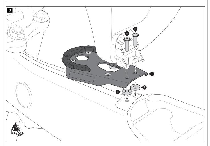
Screw the mounting bracket [4] to the seat on the vehicle. **A** WARNING: Use a liquid threadlocker!
