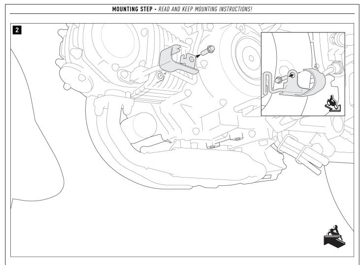
Remove the screws and cover plates shown  $\ensuremath{\mathbf{on}}\xspace$  both sides of the cylinder.
