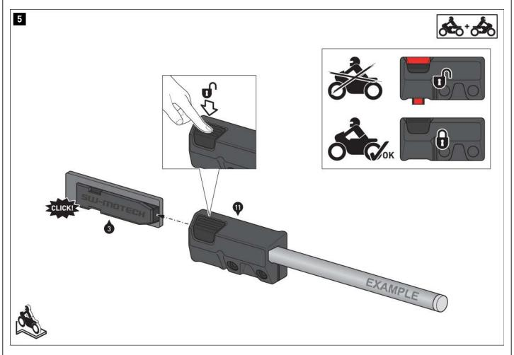
Slide the connectors (11/12) onto both sides of the connector mounting rails (3/4).
