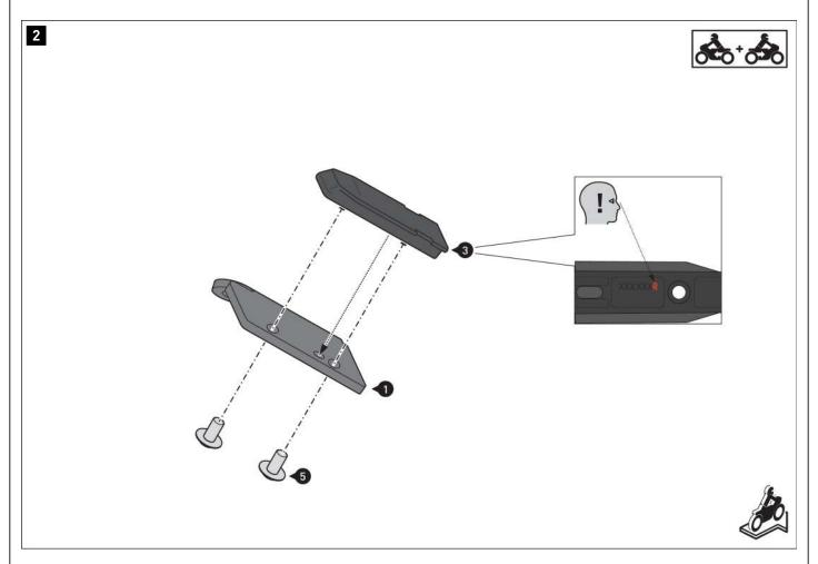
Screw the connector mounting rail (3) to the **R mark** on the mounting bracket (1).
