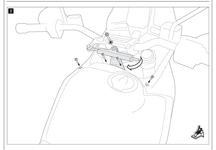
Remove the original screw of the handlebar damper.  $\triangle$  **NOTE:** Make sure that all other components such as the flanged spacers and sealing rings remain in position.
