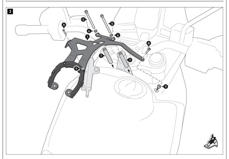
Screw the mounting bracket (1) to the vehicle.
