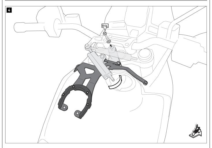
Screw the handlebar damper back onto the handlebar damper mount. Tighten the original screw (Orig.) according to the vehicle manufacturer's specifications.
