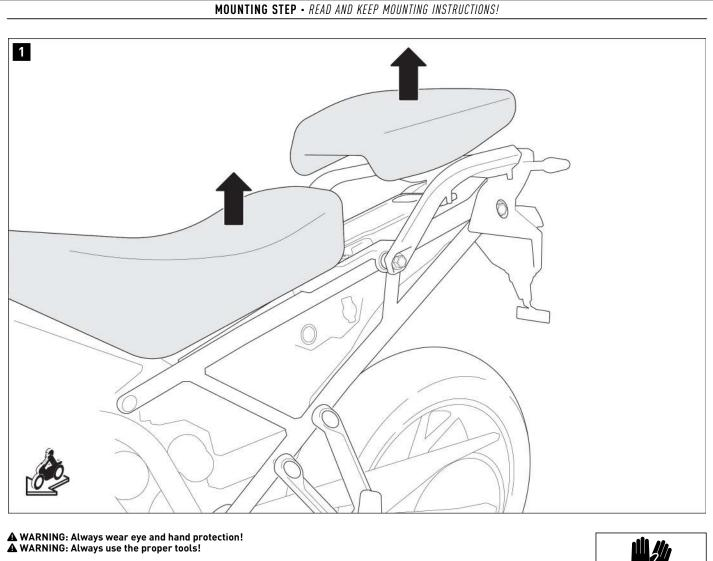
Remove the passenger seat and seat from the vehicle. In vehicles with heated seats, the connector on the seat must be removed.
