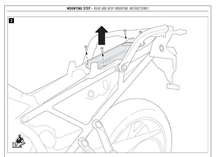
Remove the screws shown, loosen the connector, and remove the control unit with the cover from the vehicle.
