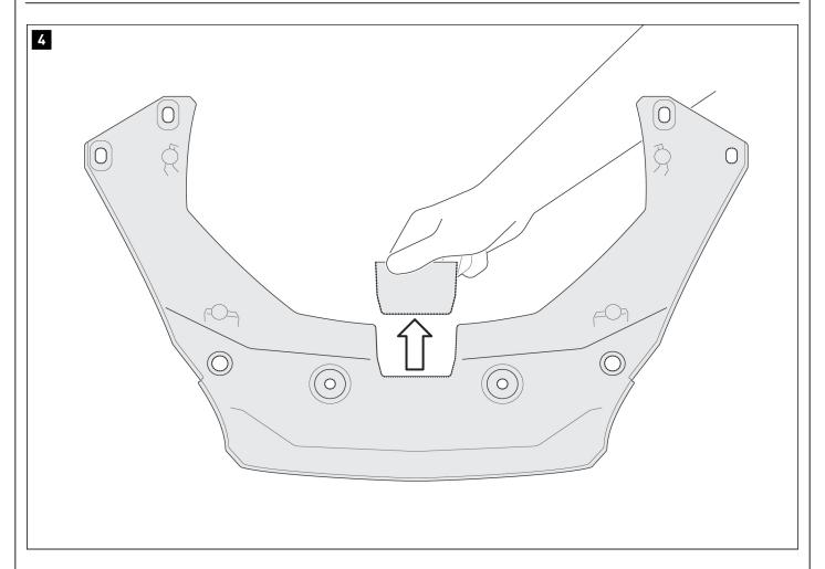
Carefully detach the pre-perforated part from the headlight cover.
