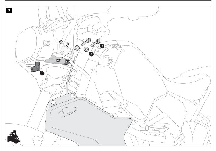
Screw the mounting bracket (1) on the left side of the vehicle to the inside of the steering head, between the plates (A) and (B).
