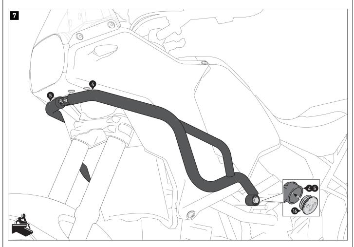
When all components are loosely attached, tighten all screws as specified in the mounting instructions.
