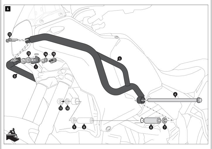
$\triangle$  **NOTE:** If the crash bars are installed at the same time as the SW-MOTECH engine guard, the spacers (7) and (9) are not required.
