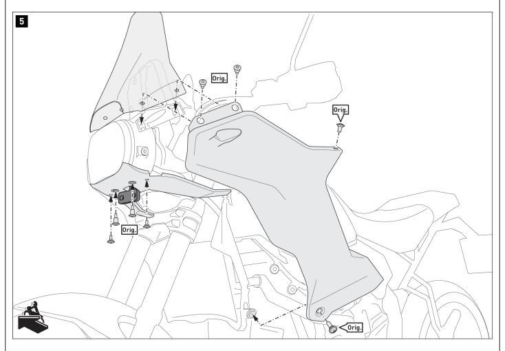
Reattach the previously disassembled trim parts to the vehicle.
