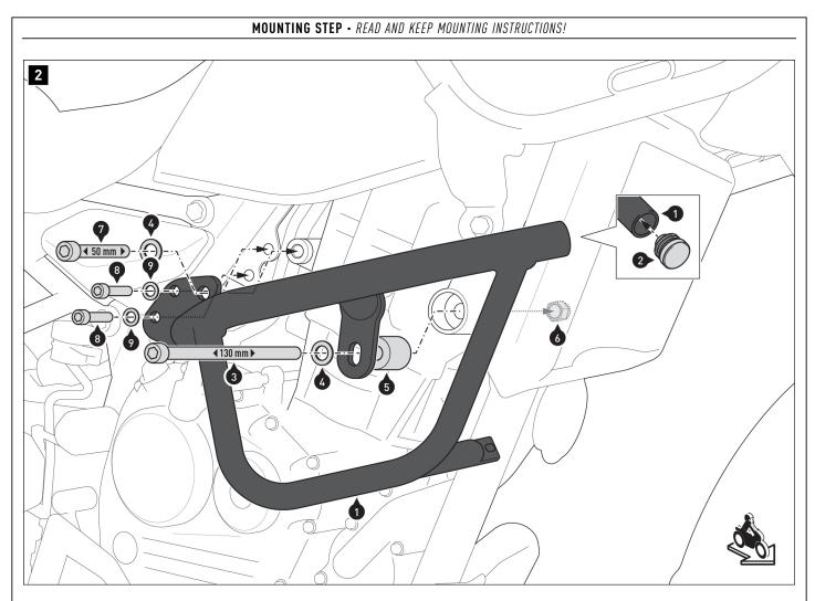
Insert the plastic plug (2) into the opening of the **right** crash bar (1).
