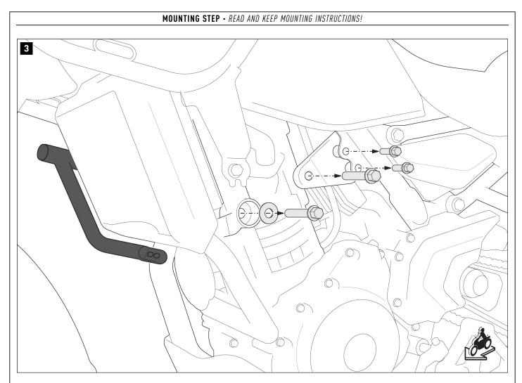
Remove the original screws from the mounting points shown on the  ${\bf left\ side}$  of the vehicle.
