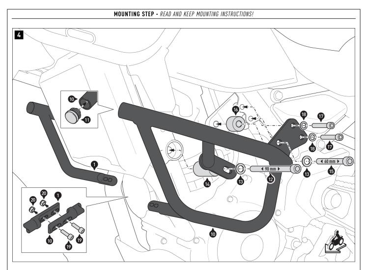
Insert the plastic plug (11) into the opening of the **left** crash bar (10).
