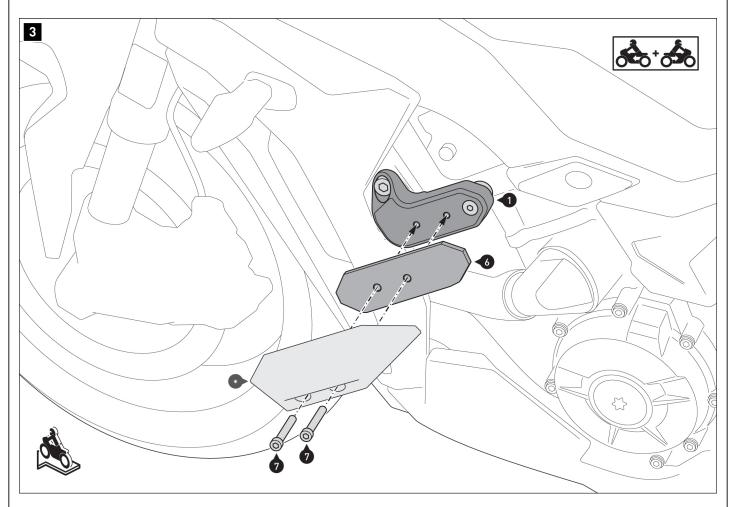
Screw the parts shown onto the screw plates [1/2].
