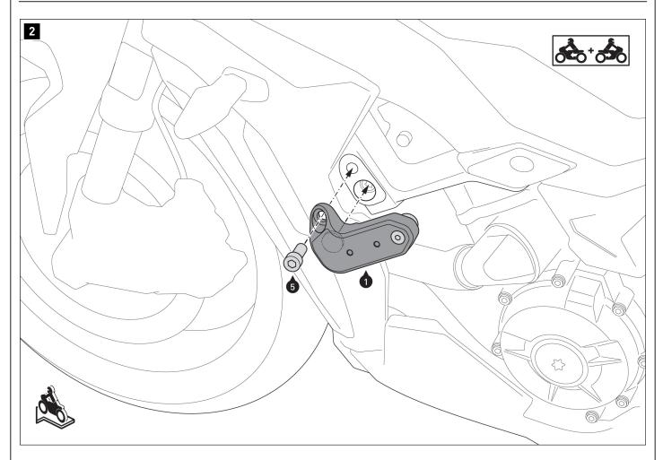
Mount the screw plates (1/2) on both sides of the bike. **A** WARNING: Use a liquid threadlocker!
