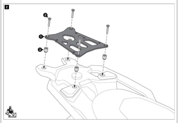
Screw the mounting bracket [1] to the mounting points shown. **A** WARNING: Use liquid threadlocker!
