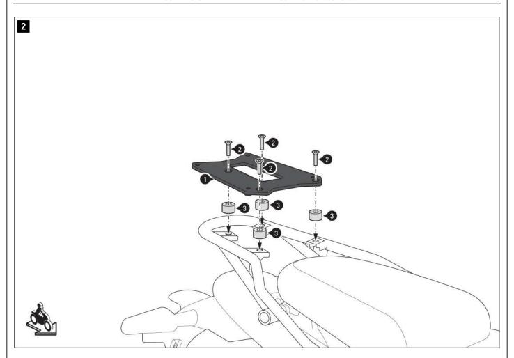
Screw the mounting bracket [1] to the mounting points shown. **A** WARNING: Use a liquid threadlocker!
